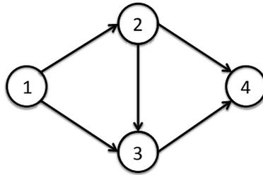
Figure 1: The graph describing the precedence constraints between the tasks in the project management problem. A directed edge from node  $i$  to node  $j$  means that task  $j$  cannot start before task  $i$  is completed (e.g.,  $i = 1$  and  $j = 2$ ).
